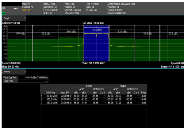
Figure 40. 80 MHz 802.11AC ACLR at 5530.0 MHz
