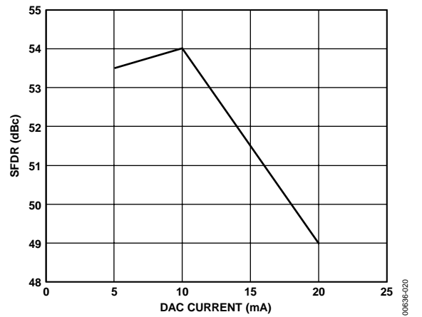
Figure 20. SFDR vs. DAC Current, 59.1 A OUT , 300 MHz REFCLK with REFCLK Multiplier Bypassed
