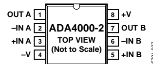
Figure 3. 8-Lead SOIC (R-8)
