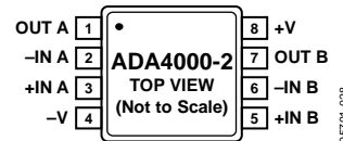
Figure 4. 8-Lead MSOP (RM-8)
