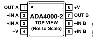
Figure 4. 8-Lead MSOP (RM-8)
