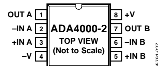
Figure 3. 8-Lead SOIC (R-8)
