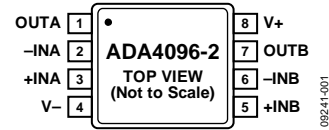
Figure 1. 8-Lead, MSOP (RM-8), ADA4096-2
