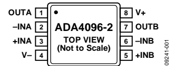
Figure 1. 8-Lead, MSOP (RM-8), ADA4096-2
