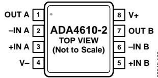
Figure 5. ADA4610-2 Pin Configuration, 8-Lead MSOP (RM Suffix)
