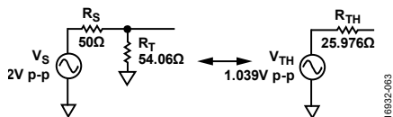
Figure 107. Thevenin Equivalent Circuit
