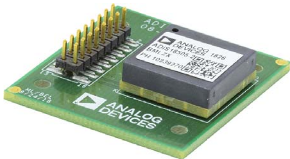
Figure 63. ADIS16505-2 Breakout Board
