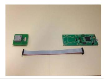
2 Install one side of the ribbon cable onto J1 of the ADIS16IMU/PCBZ
