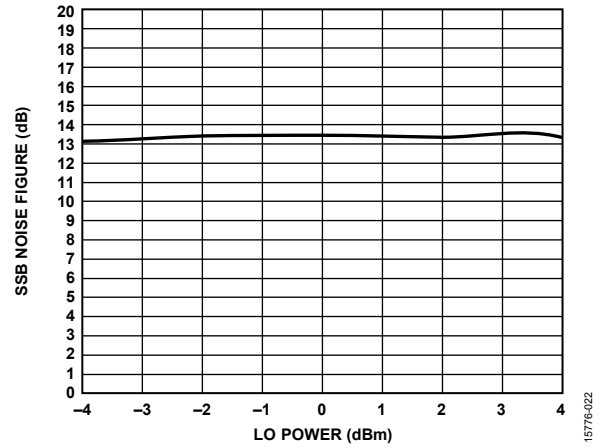
Figure 22. SSB Noise Figure vs. LO Power, RF Frequency = 23 GHz
