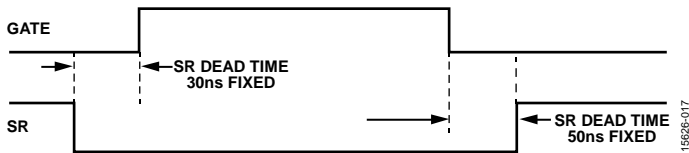
Figure 20. Gate to SR Dead Time
