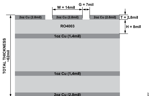
Figure 2. Evaluation Board Stack-Up
