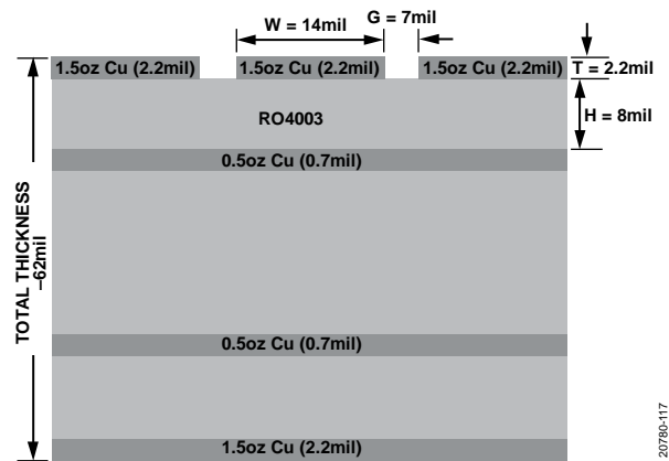
Figure 17. Probe Matrix Board Stack Up
