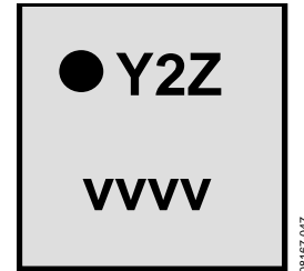
Figure 2. Product Information on Package (Top View)
