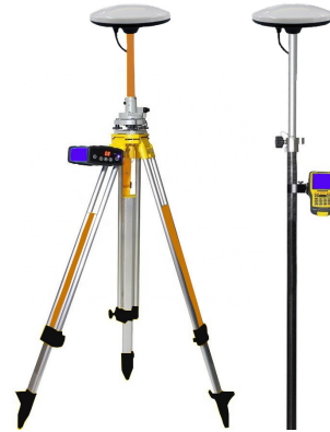
Figure 5: Surveying - The AEAGMK148060-S1575 antenna is illustrated here. However, the AEACAC055027-SG4L2 antenna can also be used.
