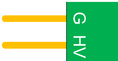
Figure 6: SiPM High Voltage Connector Detail
