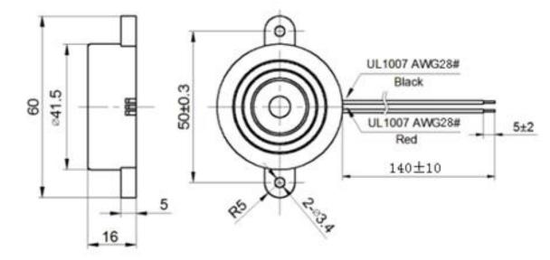
Dimensions (All dimensions in mm, tolerance ±0.5mm unless otherwise noted)
