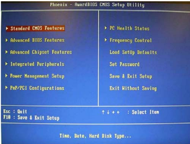
Figure 2.1: Award BIOS Setup initial screen
