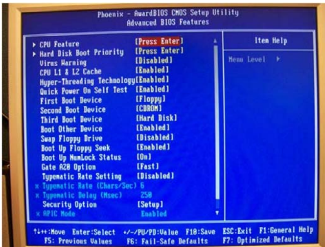
Figure 2.3: Advanced BIOS features screen
