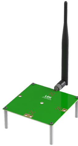
Figure 10. 5GMWP1 on Edge of Ground Plane, Bent 90 Degrees (Edge-Bent)
