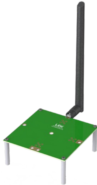
Figure 3. ANT-8/9-IPW1-SMA at Edge of Ground Plane, Bent 90 Degrees (Edge Bent)
