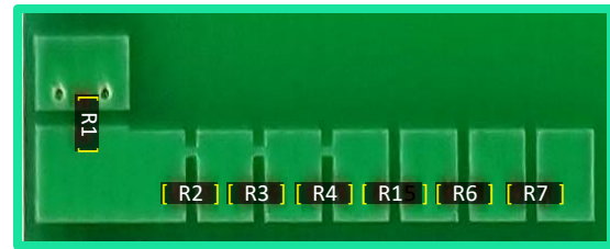
Tune Low Band Lower (Add 0Ω)
