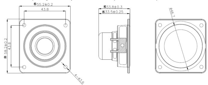
Note: Recommended speaker baffle opening is 53.5mm. Always test-fit prior to closing mechanical design.
