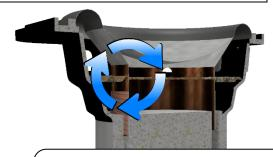
Air is forced into the magnetic loop on both sides of the voice coil for improved heat dissipation
