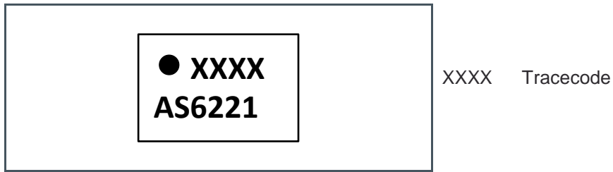
Figure 39: WLCSP Package Marking/Code for AS6221
