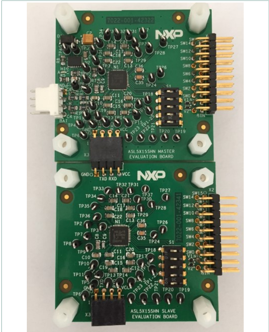
Figure 1. Connection between master and slave evaluation boards
