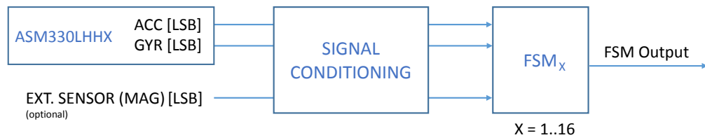
Figure 2. State machine in the ASM330LHHX
