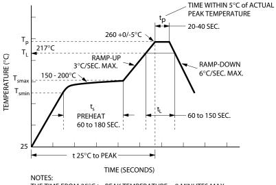
THE TIME FROM 25°C to PEAK TEMPERATURE = 8 MINUTES MAX.  $T_{smax}$  = 200°C,  $T_{smin}$  = 150°C
