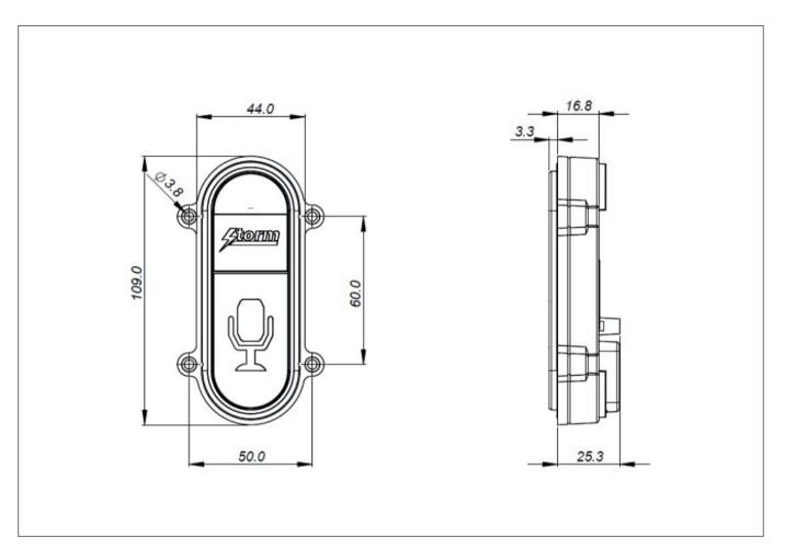
The Storm ATP Microphone Activation Sensor is a USB peripheral device that includes an internationally recognised microphone icon to indicate the presence of a voice recording device. The illuminated microphone icon is both highly visible and tactilely discernible.
