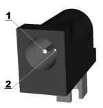
You should apply 9 VAC or +12VDC on pin 1.
