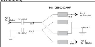
Figure 1 The Balun with external capacitors on both low impedance ports (nominal/test configuration). The two capacitors improve the insertion loss and return loss in the 40-200MHz range over that of the basic balun.
