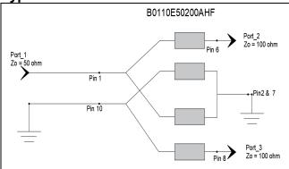
Figure 2 The Balun in it's basic configuration with no external components.
