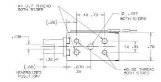
Solenoid shown energized with plunger fully seated
