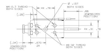
Solenoid shown energized with plunger fully seated
