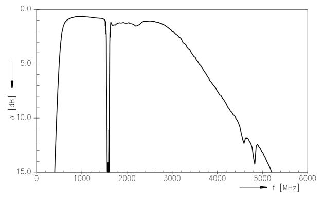
**GPS-CELL** (isolation, transfer function)
