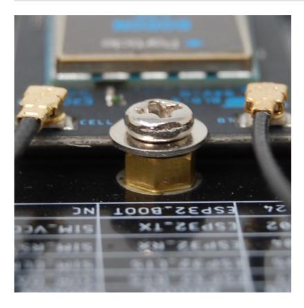
We recommend this screw assembly to securely affix the B series SoM to your circuit board. From top to bottom:
