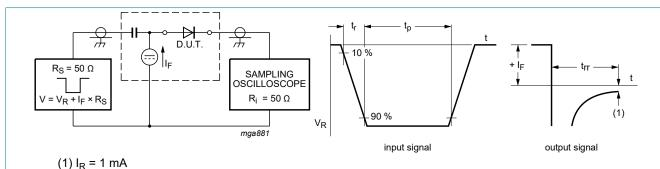
Input signal: reverse pulse rise time  $t_r$  = 0.6 ns; reverse voltage pulse duration  $t_p$  = 100 ns; duty cycle  $\delta$  = 0.05 Oscilloscope: rise time  $t_r$  = 0.35 ns
