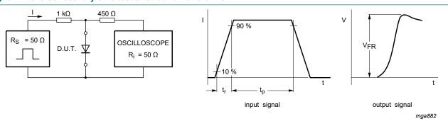
Input signal: forward pulse rise time  $t_r$  = 20 ns; forward current pulse duration  $t_p \ge 100$  ns; duty cycle  $\delta \le 0.005$
