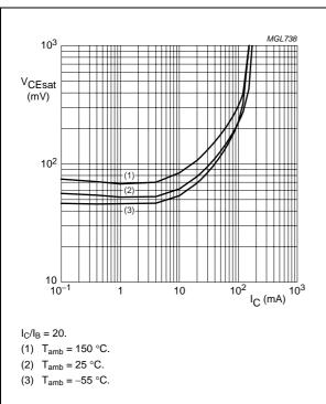
Fig.2 Collector-emitter saturation voltage as a function of collector current; typical values.
