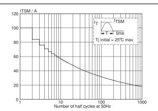
Fig.4. Maximum permissible non-repetitive peak on-state current  $I_{\text{TSM}}$ , versus number of cycles, for sinusoidal currents, f = 50 Hz.
