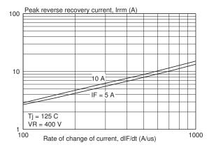
Fig.8. Typical peak reverse recovery current, I<sub>rm</sub> as a function of rate of change of current dI<sub>F</sub>/dt.
