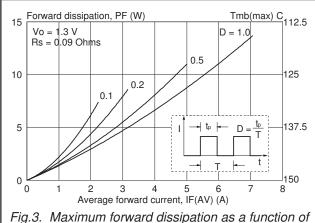
Fig.3. Maximum forward dissipation as a function of average forward current; rectangular current waveform where I<sub>F(AV)</sub> =I<sub>F(RMS)</sub> x √D.
