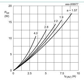
a = form factor =  $I_{F(RMS)}/I_{F(AV)}$ Vo = 1.268 V; Rs = 0.031  $\Omega$
