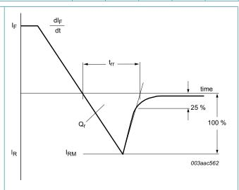
Fig. 7. Reverse recovery definitions; ramp recovery
