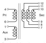
Secondary windings to be connected in parallel on PC board.
