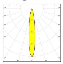
Dimensions: 21.6 mm x 21.6 mm Height: 11.70 mm ~10° diffused spot beam optimized for LUXEON Rebel ES
