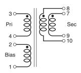
Secondary windings to be connected in parallel on the PC board
