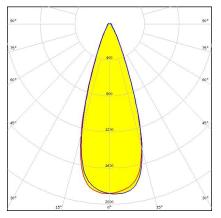
Dimensions: 69.8 mm x 69.8 mm Height: 29.90 mm ~35° medium beam compatible with 3rd party connectors from BJB, Stucchi and Tridonic
