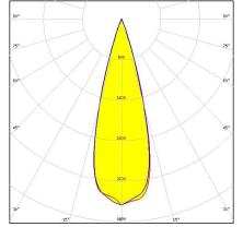
Dimensions: 69.8 mm x 69.8 mm Height: 23.60 mm ~35° medium beam
