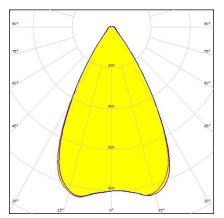
Dimensions: 69.8 mm x 69.8 mm Height: 22.10 mm ~60° wide beam compatible with 3rd party connectors from BJB, Stucchi and Tridonic
