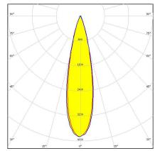
Dimensions: 69.8 mm x 69.8 mm Height: 24.80 mm ~25° spot beam
