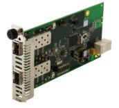
The ION C3100 is a fiber to fiber media converter module. It is protocol independent and supports data rates from 100Mbps to 2.5Gbps through two open SFP slots. This any-rate to same-rate converter can be used to perform reliable and cost-effective single mode to multimode fiber conversion or it can be used to provide wavelength conversion in CWDM applications. The ION C3100 is a manageable device when installed in a managed ION chassis.
