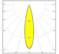
Dimensions: 35.0 mm x 35.0 mm Height: 16.40 mm ~25° medium beam
