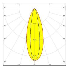
**Dimensions: 37.7 mm x 37.7 mm Height: 17.20 mm** ~40° x 15° oval beam. Assembly with holder including location pins and installation tape.
