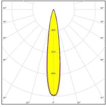
Dimensions: 35.0 mm x 35.0 mm Height: 16.40 mm ~13° spot beam
