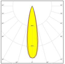
Dimensions: 37.7 mm x 37.7 mm Height: 17.20 mm ~16° diffused spot beam optimized for LUXEON M and MX. Assembly
