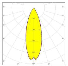
Dimensions: 35.0 mm x 35.0 mm Height: 16.40 mm  $\sim$ 40° wide beam
