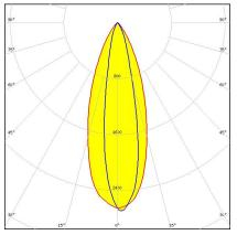
**Dimensions: 37.7 mm x 37.7 mm Height: 17.20 mm** ~40° x 15° oval beam optimized for LUXEON M and MX. Assembly with holder and installation tape.
