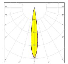
Dimensions: 35.0 mm x 35.0 mm Height: 16.40 mm ~16° diffused spot beam
