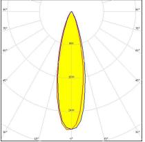
Dimensions: 37.7 mm x 37.7 mm Height: 17.00 mm ~25° medium beam optimized for
