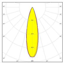
Dimensions: 37.7 mm x 37.7 mm Height: 17.20 mm ~25° medium beam. Assembly with holder including location pins and installation tape.
