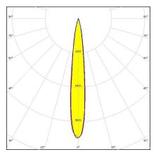
Dimensions: 35.0 mm x 35.0 mm Height: 16.40 mm ~14° smooth spot beam
