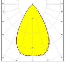
Dimensions: 37.7 mm x 37.7 mm Height: 17.20 mm ~55° wider beam. Assembly with holder including location pins and installation tape.
