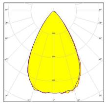
Dimensions: 37.7 mm x 37.7 mm Height: 17.00 mm ~55° wide beam optimized for LUXEON M and MX. Assembly with holder and installation tape.
