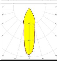
LED MJT 3030  $\mathsf{FWHM}\,/\,\mathsf{FWTM}$ 33.0° / 66.0° Efficiency 96 % Peak intensity 2.3 cd/lm LEDs/each optic 1 Light colour White
