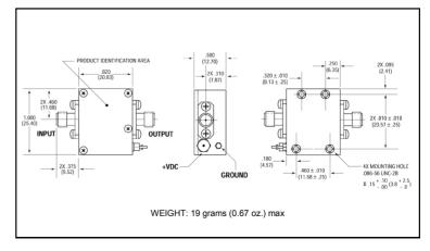
\* Dimensions are inches (millimeters) ±0.015 (0.38) unless otherwise specified.
