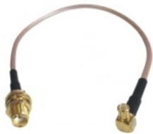
SMA FEMALE-RG174-MCX (M) R/ANGLE 200MM LONG
