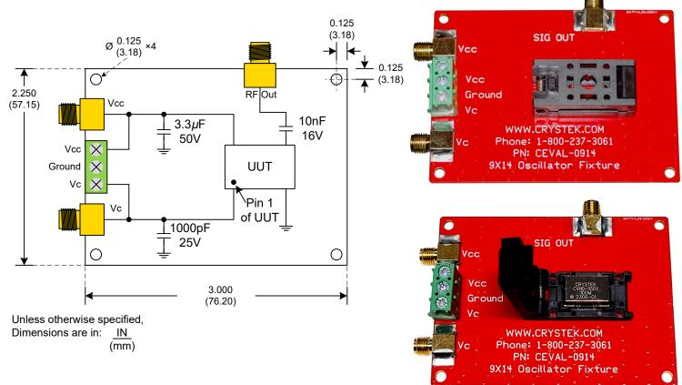
Features: Connectors: Gold Plated SMA Female Connectors Frequency Range: up 3 GHz PCB: 0.062" FR4 Operating Temperature: -40°C to +85°C
